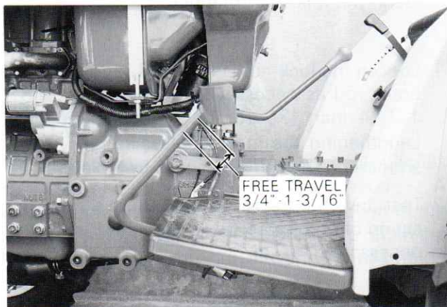
Figure 59 – Clutch Pedal Free Travel Adjustment
